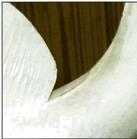
The cutting disc leaves only a tiny bit of flashing to sand away. A BIG time savings.
