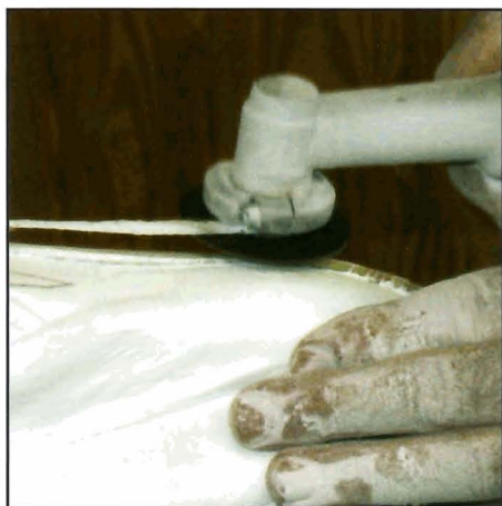
Cutting flashing to within 1/16 in. is easy, and even closer is possible if you're brave!
