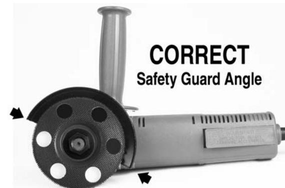
THE MAIN CRITERIA IS THAT THE BOTTOM OF THE SAFETY GUARD MUST BE AS LEVEL AS POSSIBLE WITH THE BOTTOM OF THE BODY OF THE DISC GRINDER.
